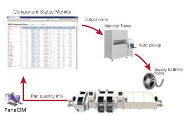
No waiting for parts to be supplied due to "No Parts"! Realize Reduce labor resources and Productivity improvement! **2**Component Supply Navigator
