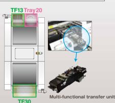
13 fixed feeder slots are available. PoP tray mounting is possible via a transfer unit.
