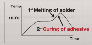
After the solder melts, self-alignment and component sinking occurs.
