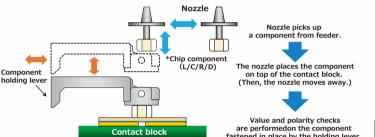
At the start of production, or during component supply or product changeover, it checks mounted component values. This helps improve machine availability through a reduction in time spent on component checks, as well as preventing misplacement due to loading of components on wrong feeder, defective components, or mislabeled reels, and thereby contributes to manufacturing conforming items.
